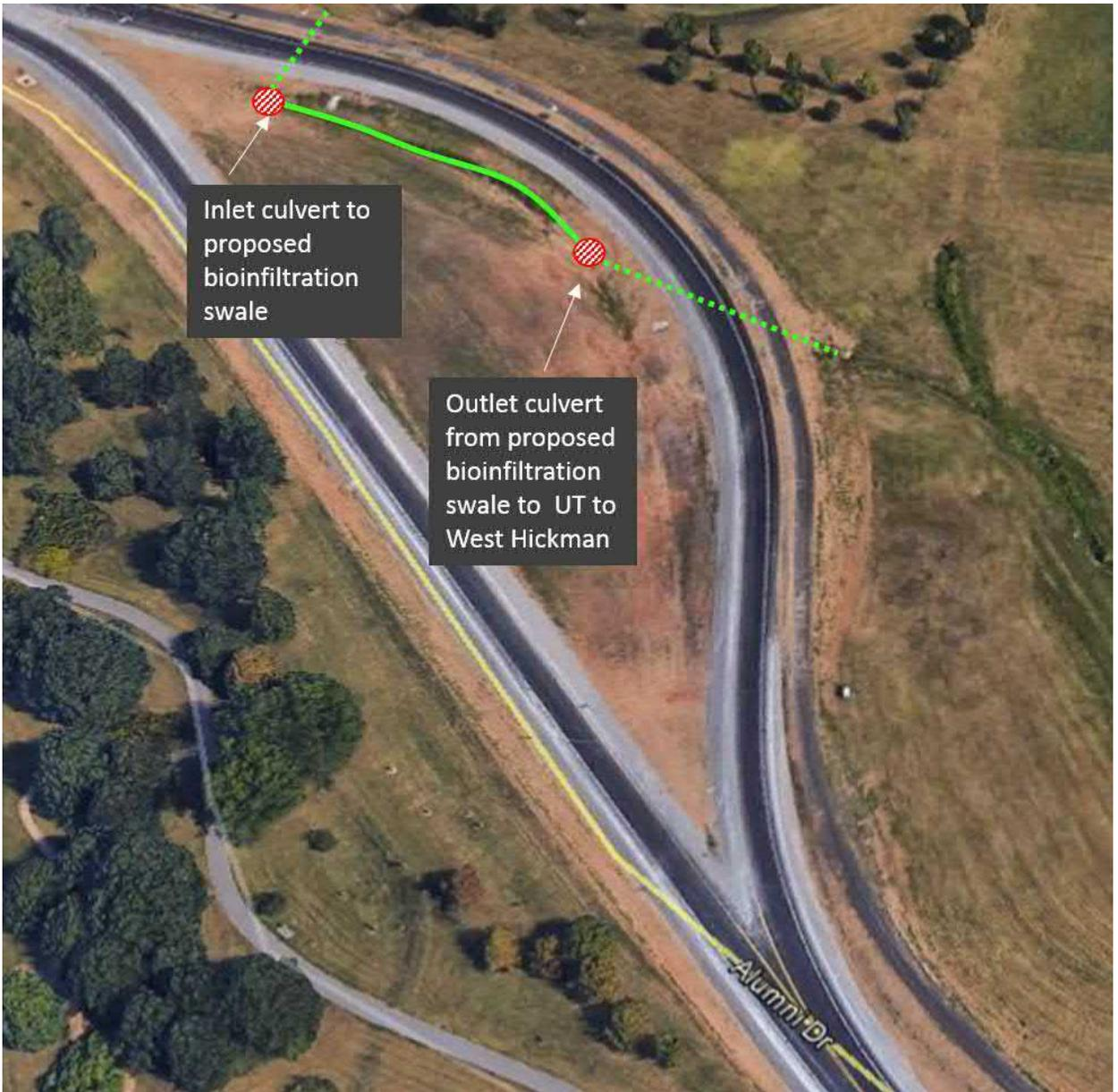
Figure 3. A portion of the flow passes under Alumni Drive (dashed green line at top of figure), enters a traffic island basin, and then passes under Alumni Drive again (second dashed green line from basin outlet) before entering the UT to West Hickman. The solid green line represents the proposed bioinfiltration swale.
