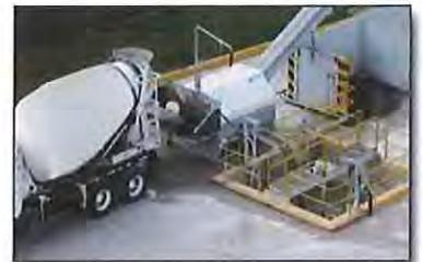
**Figure 5.** Ready mixed truck washing out into a reclaimer
