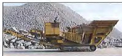
**Figure 6.** Crushed concrete stockpile and crusher
