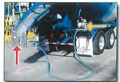
Figure 8. Chute washout bucket and pump
