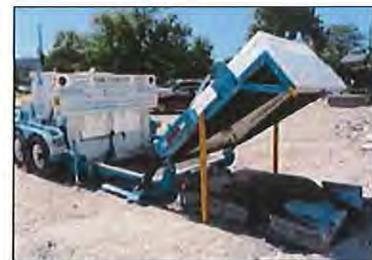
Figure 17. Delivering hardened concrete to a recycler
