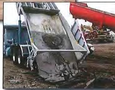
Figure 15. Delivering hardened Concrete to a recycler
