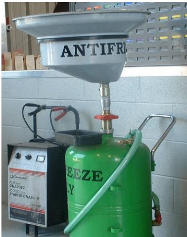
Antifreeze that contains more than 5 mg/l (ppm) TCLP lead must be managed as a hazardous waste.
